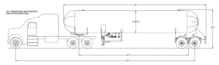
**CHASSIS FRAME** – Steel welded to tank frame
